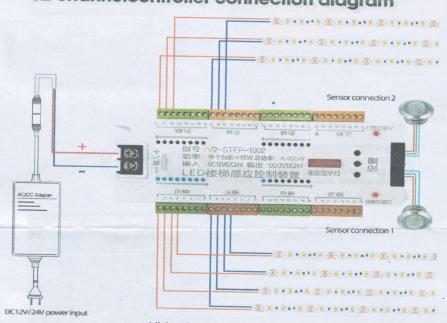
A light strip needs to insert the positive pole in the orange port 1 and the negative pole in the green port 1.
