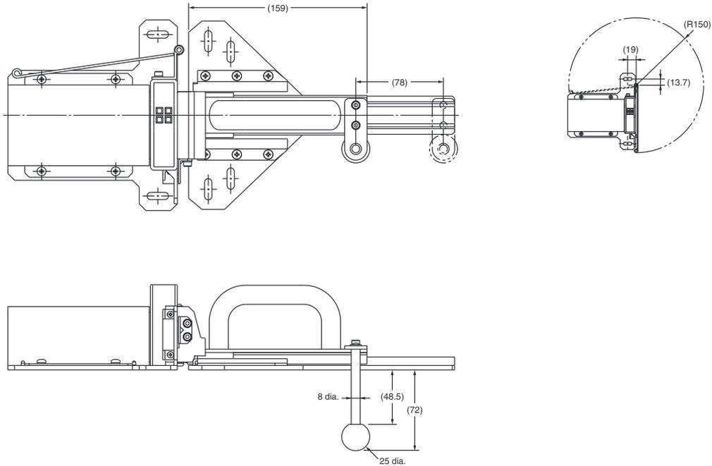
With Operation Key Inserted (Relationship between Insertion Radius and Key Hole)
