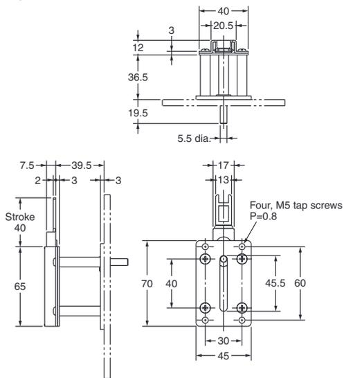
Auxiliary Mounting Bracket and Receptacle Bracket
